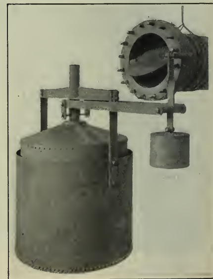
FIG. 10. GASOMETER PRESSURE REGULATOR SHOWING METHOD OF OPERATING BUTTERFLY IN GAS INLET
